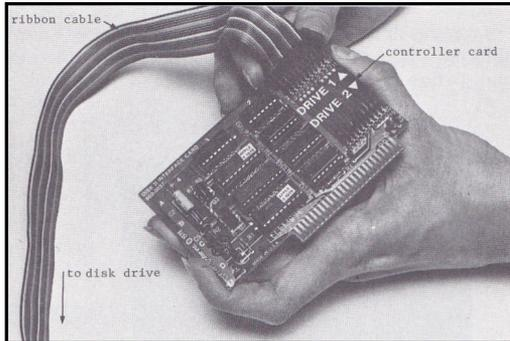
" Connecting the Cable to the Controller "
