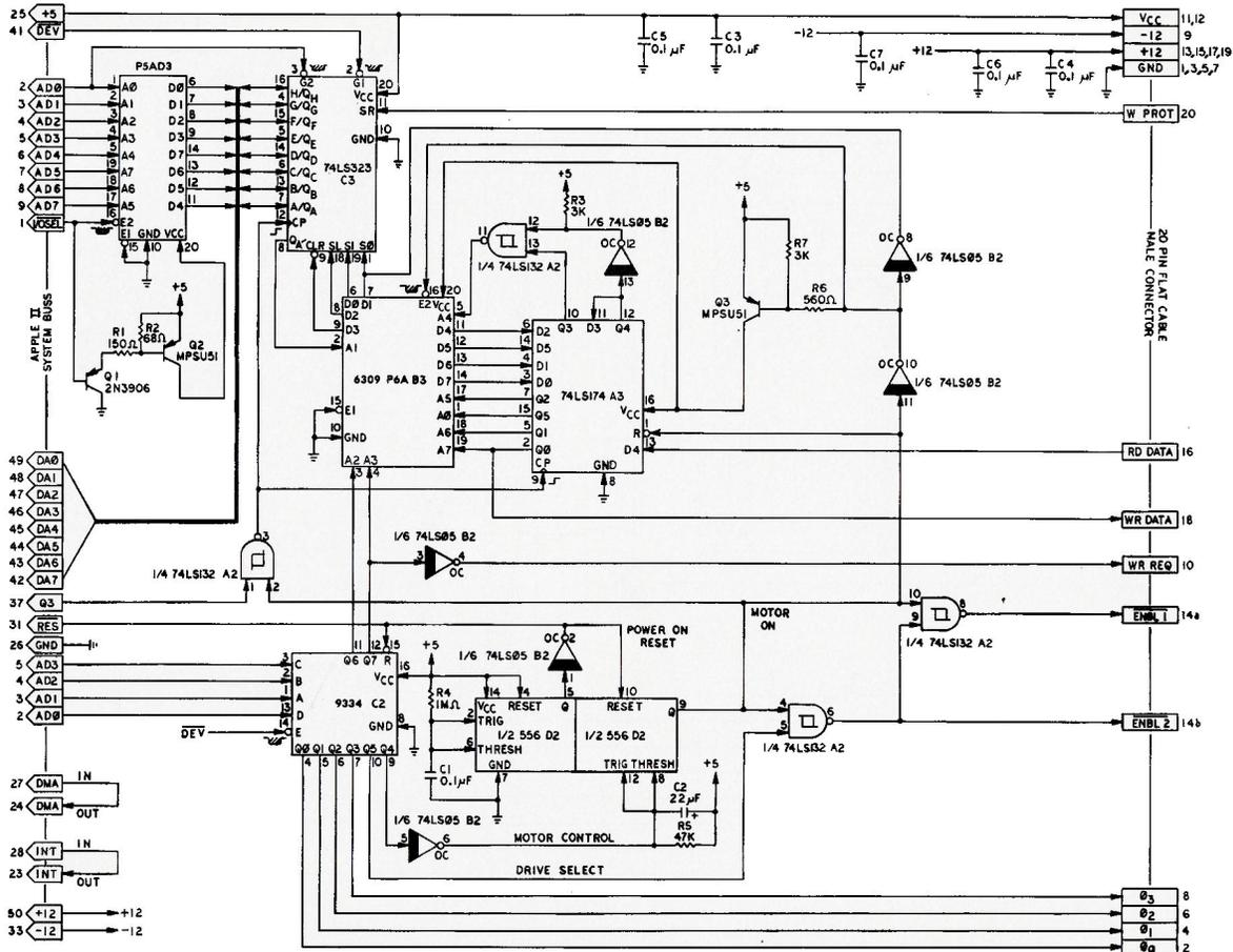
CIRCUIT SCHEMATIC: DISK II INTERFACE
